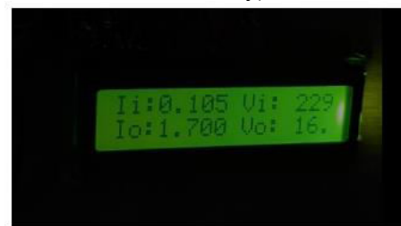
Notification through buzzer at set threshold (1.70 Amp)
